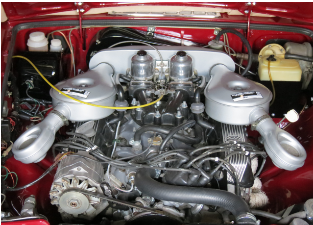
Refurbished air cleaners – new valve on the left
