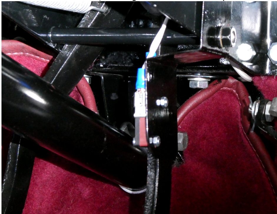
Microswitch in place and connected up
